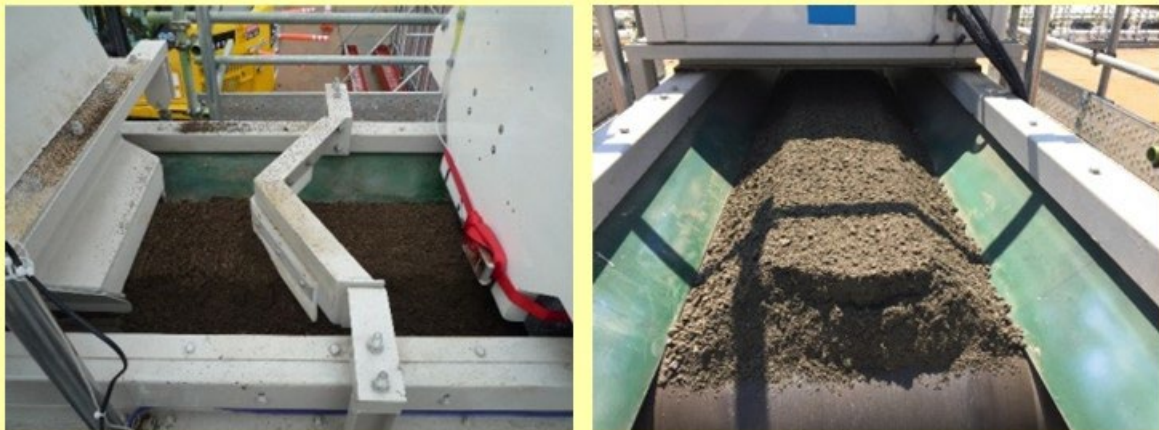
Fig.2-5 Radioactivity concentration measuring equipment using a conveyor belt
