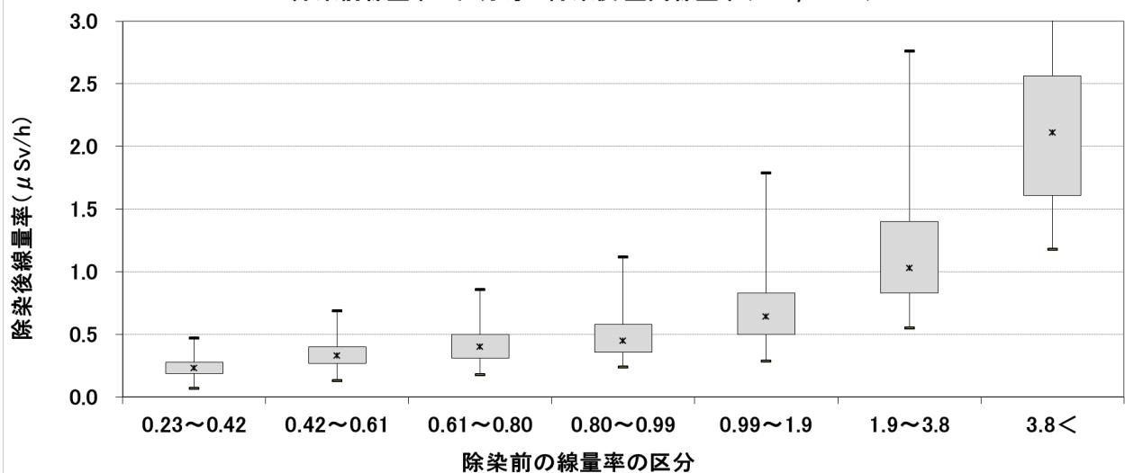
除染前線量率の区分毎の低減率 ( $1\text{m} : \mu\text{Sv}/\text{h}$ )
