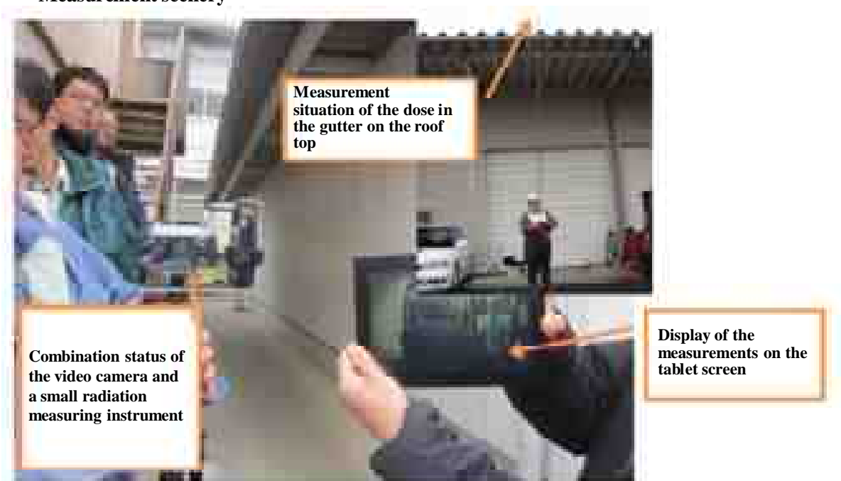
Figure 1-10 A good practice: Measurement of air dose rates in high places such as rooves and rain gutters 43 .
