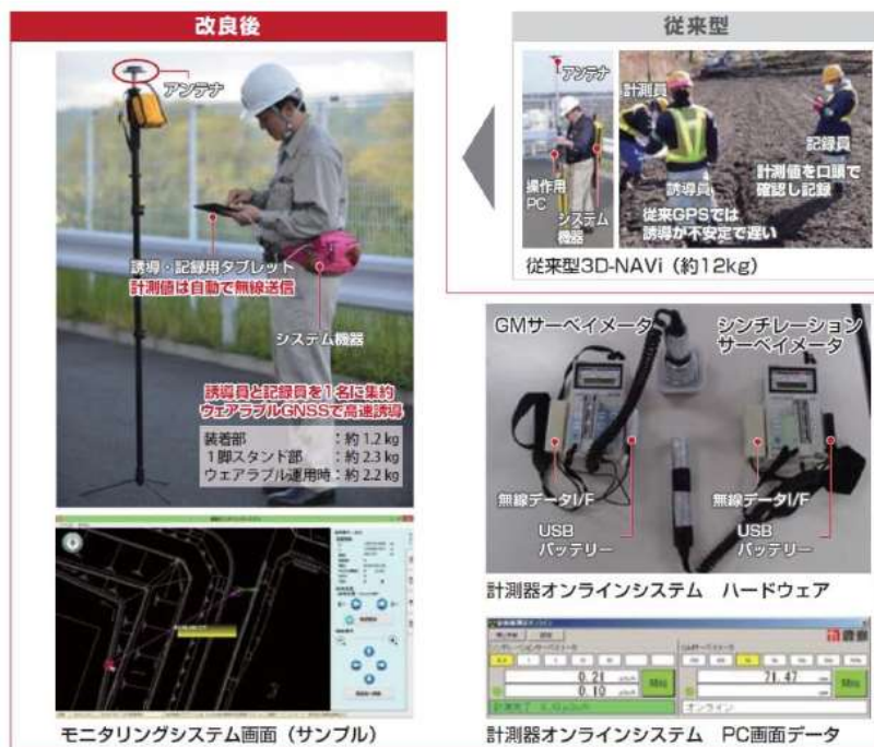
Figure 4-8 Example of an air dose rate measurement system with a wearable Global Navigation Satellite System
