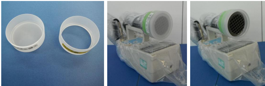
Figure 1-19. Example of a Plastic Shield Plate and Spacer (Left) and Mounting Configuration for the Shield Plate and Spacer (Center, Right)
