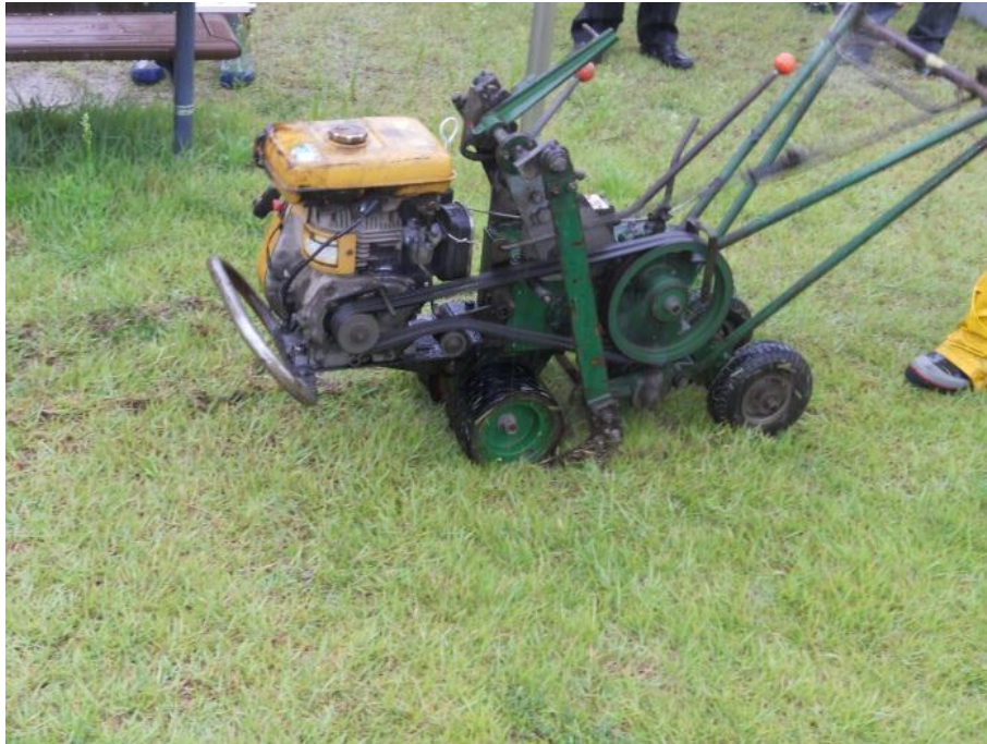
Figure 2-60. Example of decontamination work for a lawn (deep trimming)
