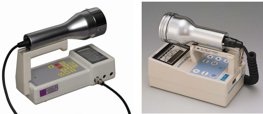
Figure 1-8. Examples of GM Survey Meters
