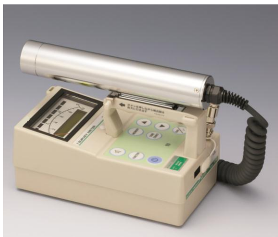
Figure 1-7. Examples of Scintillation Survey Meters (NaI scintillation survey meters)
