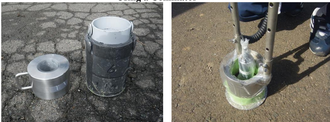
Figure 1-12. Example of a Collimator (Left) and an Example of Measurements Using a Collimator
