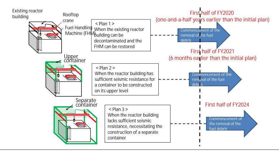
Future plans will be narrowed down in the first half of FY2014 based on the results of analysis of the likelihood of the existing reactor building's decontamination or restoration of the FHM, as well as the results of the assessment of the seismic resistance of the existing reactor building.
