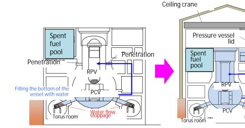
Rough picture of the process from repairing the bottom of the RCV (water flow stoppage) to filling the bottom of the vessel with water
