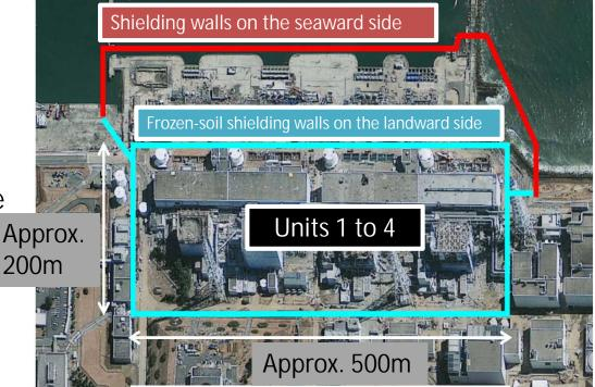
[Plan to construct shielding walls on the landward side]
