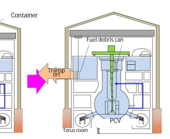
Rough picture indicating the process of removing the fuel debris
